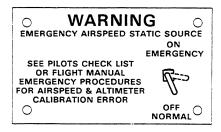
On Lower Sidewall Adjacent To Pilot: (TC-1403 thru TC-1607 - STANDARD)
