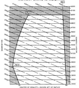
ENVELOPE BASED ON THE FOLLOWING WEIGHT AND CENTER OF GRAVITY LIMIT DATA (LANDING GEAR DOWN)
