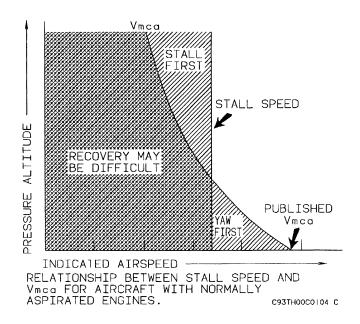
Engine-out minimum control speed generally decreases with altitude, while the single engine stall speed remains approximately constant for normally aspirated engines. No such demonstration should be attempted when the altitude and temperature are such that the engine-out minimum control
