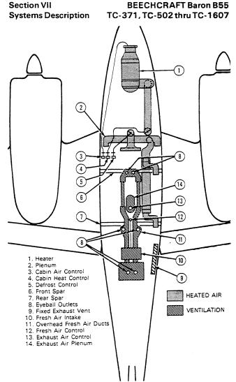
HEATING AND VENTILATION SYSTEM SCHEMATIC TC-371, TC-502 THRU TC-954
