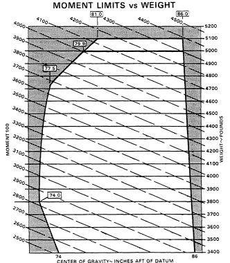
ENVELOPE BASED ON THE FOLLOWING WEIGHT AND CENTER OF GRAVITY LIMIT DATA (LANDING GEAR DOWN)
