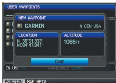
New Waypoint Window (POSITION Softkey Selected) (Split-Screen)
