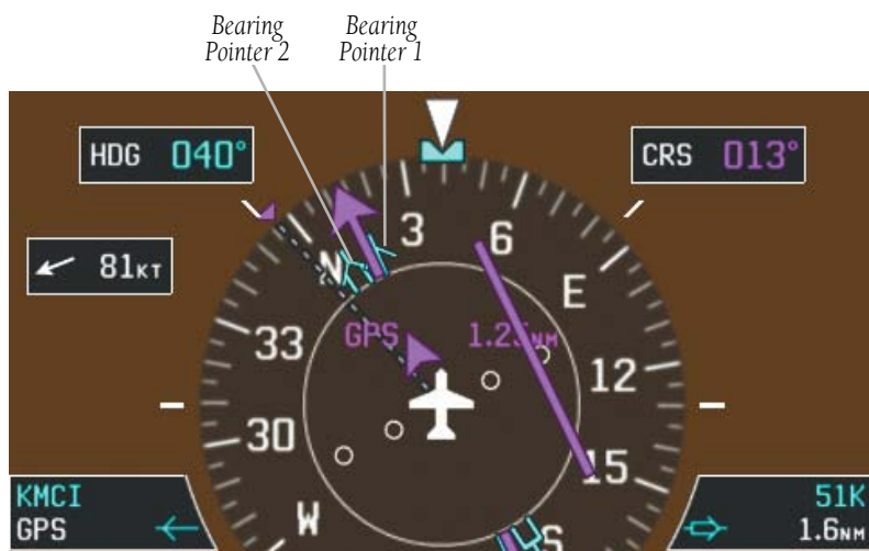
Bearing 1 Information Window -Identifier -Bearing Source
