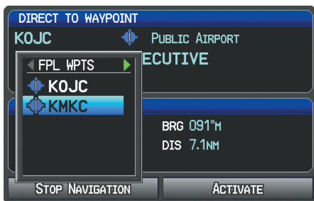
Direct-to Window (Flight Plan Waypoints Selected) (Single Display)
