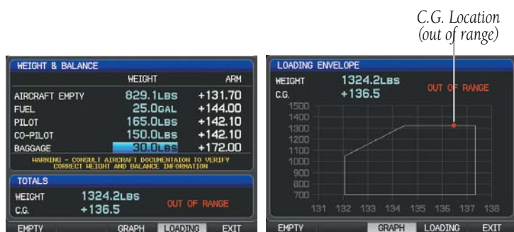
Weight & Balance Page (C.G. Out of Range) (Single Display)
