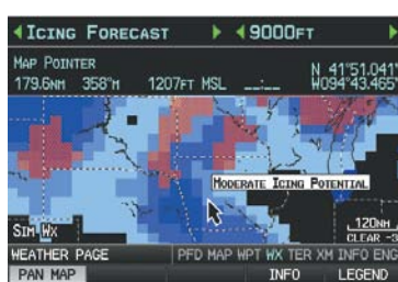
Moderate Icing Selected With Map Pointer (Single Display)
