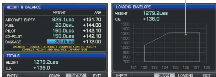
Weight & Balance Page (C.G. in Range) (Single Display)
