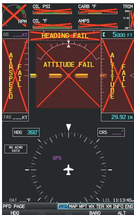
G300 System Failure Annunciations (Single Display)
