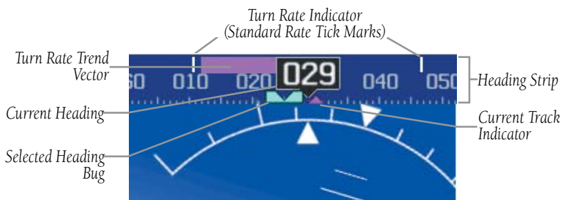
Heading Strip/Turn Rate Indicator
