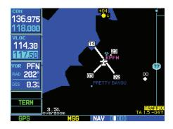
Turn the small left knob to select the desired kilohertz (kHz) value. For example, the '.70' portion of the frequency '117.70'.
