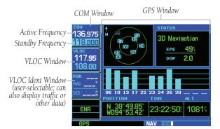
Each unique screen of information is referred to as a page. Pages are typically selected using the small and large **right** knobs, with the cursor removed from the GPS Window. See pages 6 and 7 for details on arrangement of the GNS 530's main pages.
