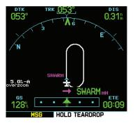
4) The GNS 530 provides course guidance only on the inbound side of the holding pattern. When leaving the holding pattern to re-fly the approach (or another approach) press the **PROC** Key to 'Select Approach?' or 'Activate Approach?' as previously described. Or, use the **Direct-to** Key to select another destination.
