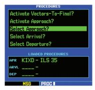
A window appears listing the available procedures. Turn the large right knob to highlight the desired procedure and press the ENT Key.
