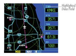
Turn the small **right** knob to select the desired type of data for this field and press the **ENT** Key.
