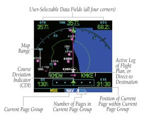
The following symbols are used on the Default NAV Page (directly above the CDI), to depict the 'active leg' of a flight plan or direct to:
