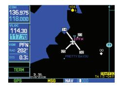
To activate the selected frequency, press the COM Flip-flop Key for COM frequencies, or the VLOC Flip-flop Key for VLOC frequencies.
