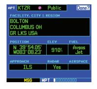
3) To view additional WPT pages for the selected airport (including the airport runway and airport frequency pages), press the small **right** knob to remove the flashing cursor. Turn the small **right** knob to display the additional WPT pages. When finished, press the small **right** knob to return the flashing cursor to the display.
