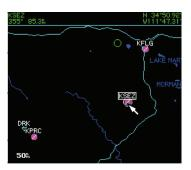
If the panning pointer is placed on an open location, press the **Direct-to** Key then press the **ENT** Key twice to create a '+MAP' waypoint and navigate to it.
