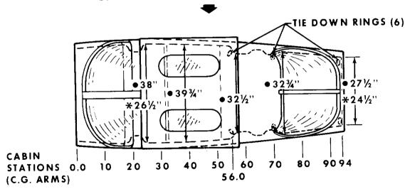
Figure 6-5. Internal Cabin Dimensions
