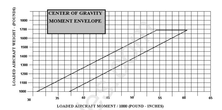
Figure 6-8 Center of Gravity Moment Envelope
