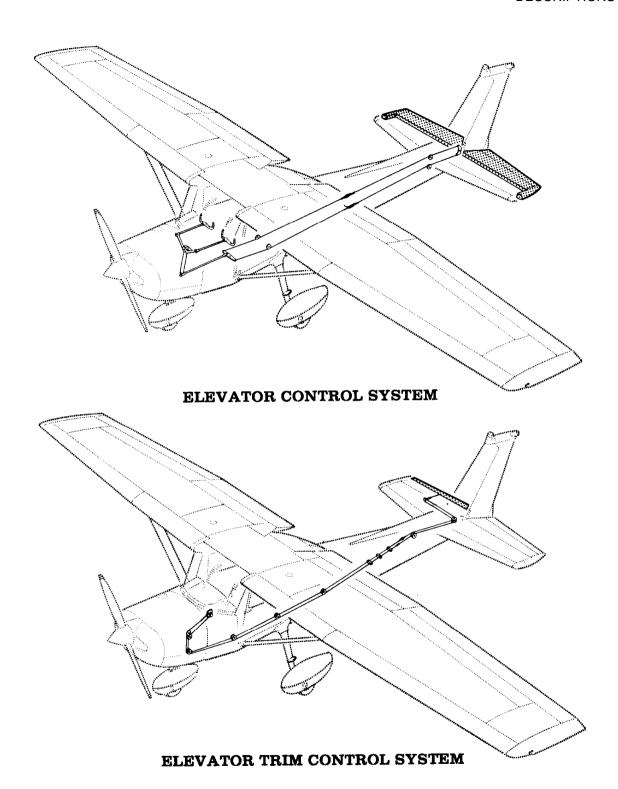
Figure 7-1. Flight Control and Trim Systems (Sheet 2 of 2)
