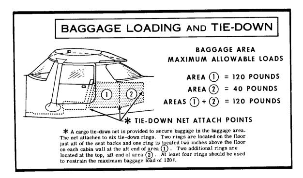
Figure 6-4. Baggage Loading and Tie-Down
