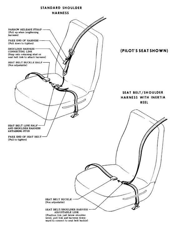
Figure 7-4. Seat Belts and Shoulder Harnesses
