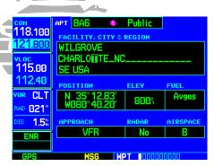
When selecting a waypoint by facility name or city, you can scroll through duplicate entries by continuing to rotate the **small right knob**.
