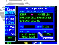
Confirm the selected direct-to destination by highlighting "Activate?" and pressing **ENT**.
