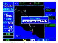
STEP 2 & 3: From the Airport Departure Page, press **MENU** to display an options list. "Load into Active FPL?" allows you to add the arrival procedure to the beginning of your flight plan.
