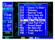
The **large right knob** is used to select the data field you wish to change. Then use the **small right knob** to display a list of data options and select the desired data item
