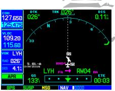
STEP 13: As you cross the missed approach point, "SUSP" appears on-screen above the **OBS** key. Press the **OBS** key to provide navigation guidance to the missed approach holding point.
