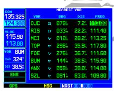
STEP 3 & 4 (top): To automatically tune a VLOC frequency, highlight the desired frequency on the VOR or Nearest VOR Pages, and press **ENT**.
