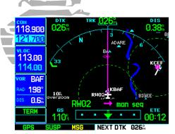
STEP 2: As you depart the airfield, "NEXT DTK 026°" appears in the lower right corner and "SUSP" appears above the **OBS** key. Indicated distance increases and is FROM the waypoint fix.
