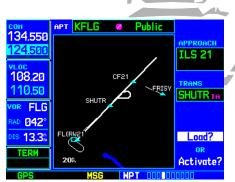
When an ILS approach is first selected, the ILS frequency is automatically placed in the standby VLOC frequency field. Press the **VLOC flip-flop key** to use this frequency.
