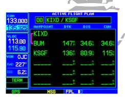
Active Flight Plan Page with flight plan currently in use.
