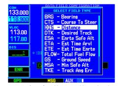
STEP 4: If "Configurable Data Fields" is selected, a second field appears to select the desired navigation data type. Rotate the **large right knob** to select this field, then rotate the **small right knob** to display the available navigation data types.
