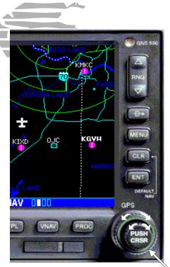
Data is entered using the **large** and **small right knobs**. Experiment with them to become efficient at entering data. This greatly reduces the amount of time spent operating the GNS 530 in flight.
