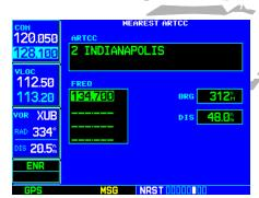
STEP 3 & 4: Rotate the **small right knob** to select the desired center, then rotate the **large right knob** to highlight the desired frequency.
