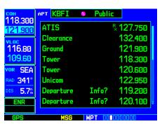
To view a different WPT page, the on-screen cursor should not be visible. (Press the **small right knob** to remove the cursor, if necessary.) Rotate the **small right knob** to select the desired WPT page.
