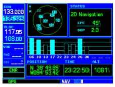
As satellites are received, the status changes to "2D Navigation" or "3D Navigation". "3D Navigation includes altitude, whereas "2D Navigation" is only the latitude/longitude position.
