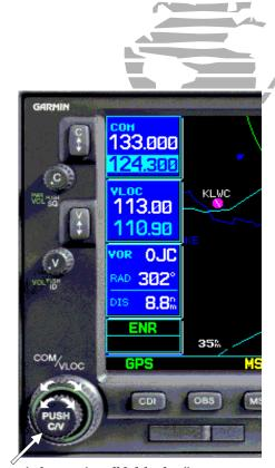
The **large** and **small left knobs** allow you to tune the desired COM or VLOC frequency.
