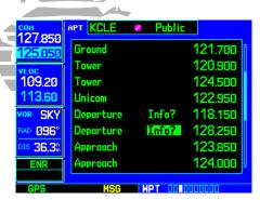
When "Info? appears to the left of a displayed frequency, the frequency has usage restrictions.
