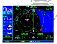
Nine map scale settings are available on the Default NAV Page — from 5.0 to 200 nautical miles. To adjust the map scale, use the **RNG** key.
