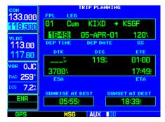
STEP 6: The current time and date are automatically offered for depature time and date. To accept either automatic selection, simply press **ENT** when the selection is highlighted.
