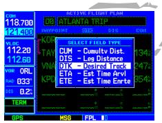
Change the displayed data using the "Change Fields?" option. Highlight the data field you wish to change and rotate the small right knob to display available data types.
