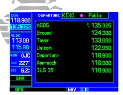
Tuning cursor in the COM window. Use the **small** and **large left knobs** to dial in the desired standby frequency.
