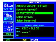
STEP 2 & 3 (bottom): When a VOR or localizer-based approach is "Loaded" or "Activated", the frequency is automatically placed in the standby field of the VLOC window.
