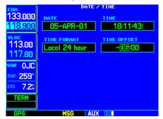
STEP 3 (bottom): Use the **small** and **large right knobs** to enter the difference between UTC (zulu) and local time.
