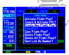
From the Flight Plan Catalog, press **MENU** to display the options menu and select "Create New Flight Plan?".
