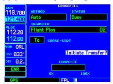
Once "Initiate Transfer?" is selected, a progress bar at the bottom of the page indicates the status of the crossfill transfer until completed.
