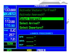
Press the **PROC** key to display the procedures page. Rotate the **large right knob** to select the desired option.
