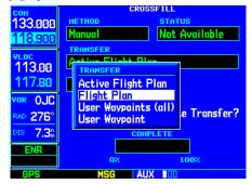
STEP 3: Rotate the **small right knob** to display a list of TRANSFER options. Continue rotating the **small right knob** to select the desired option.
