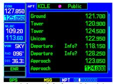
Rotate the **large right knob** to scroll through the list.
