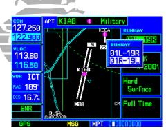
STEP 2 & 3 (top): Highlight the RUNWAY field and rotate the **small right knob** to display a listing of all runways at the selected airport.
