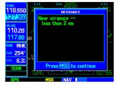
"Near airspace less than 2nm" indicates that you are within two nautical miles of an airspace, but are NOT projected to enter the airspace.
