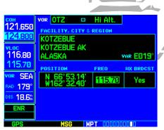
STEP 3: Using the **large right knob**, highlight the VOR's frequency and press **ENT** to place the frequency in the standby VLOC frequency field.
