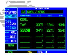
Highlight the point in the existing flight plan where you wish to add the new waypoint. If an existing waypoint is highlighted, the new waypoint is placed directly in front of it.
