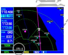
To quickly declutter the map, press **CLR**. Continue pressing **CLR** to select the desired declutter level. Note the scale is followed "-1", "-2" or "-3".
