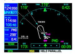
STEP 6: An alert message recommends the holding pattern entry procedure (e.g., "HOLD PARALLEL").
