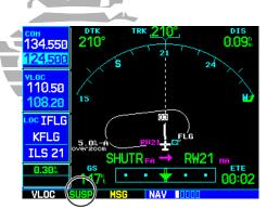
"SUSP" indicates that automatic sequencing of approach waypoints is suspended. In some instances "SUSP" automatically cancels (holding pattern entry). In other cases, press **OBS** to manually cancel
