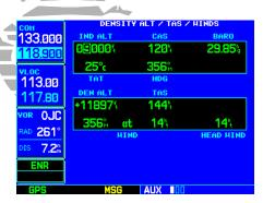
STEP 2: Use the **small** and **large right knobs** to enter the indicated altitude.
