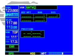
STEP 2: Use the **small** and **large right knobs** to enter a name for the new waypoint. When you press **ENT**, your present position automatically appears in the "Position" field.
