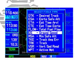
Once "Change Fields?" is selected, rotate the **large right knob** to highlight the data field you wish to change, then rotate the **small right knob** to select the type of data to display in that field.
