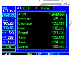
Listed communication frequencies include ATIS, clearance delivery, ground control, tower, unicom, approach and departure. The "RX" next to ATIS identifies it as a "receive only" frequency.
