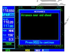
"Airspace near and ahead" indicates that you are within two nautical miles of an airspace and projected to enter the airspace.
