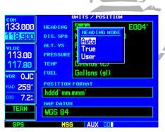
STEP 2 (top): Rotate the **small right knob** to select the desired heading mode. The default setting is "Auto", which automatically calculates the magnetic variation at your current position.
