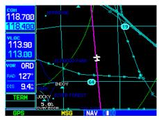
The Map Page is the second of four Nav pages (five if equipped with weather and/or traffic systems). The map scale is depicted in the lower left corner and adjusted with the **RNG** key.
