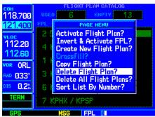
Select "Delete Flight Plan?" to remove the designated flight plan from memory.
