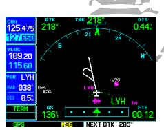
STEP 3: As you approach the IAF, the "NEXT DTK 205°" waypoint alert appears in the lower right corner. Prepare to turn to this heading.
