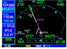
Within the shaded area of the illustration at left, the GNS 530 automatically switches the external CDI to the GNS 530's internal VLOC receiver. "VLOC" appears above the **CDI** key.
