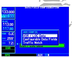
STEP 2: Rotate the **small right knob** to select the desired data field option.
