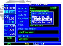
Use the Units / Position Page to switch distance and speed measurements between Nautical, Statute and Metric units.
