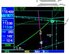
Once "Measure Dist?" is selected, place the on-screen pointer on the point you wish to measure FROM and press **ENT**.
