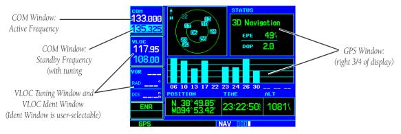
Pushing the **small left knob** moves the tuning cursor back-and-forth between the COM and VLOC frequency windows. To select the active frequency, you must first enter the frequency in the standby field, and use the **COM** (or **VLOC**) **flip-flop** key to move it to the active field.
