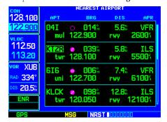
STEP 1 & 2 (bottom): You can select a direct-to destination directly from a NRST page (e.g. Nearest Airports) by highlighting the desired waypoint and pressing the **direct-to** key.
