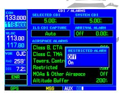
STEP 2 & 3: Rotate the **large right knob** to select the desired airspace type, then rotate the **small right knob** to select "On" or "Off".
