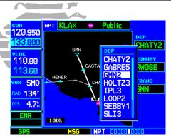
STEP 2 & 3: With the cursor on the "DEP" field, rotate the **small right knob** to display a list of available departure procedures.
