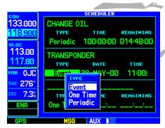
STEP 4 (top): Rotate the **small right knob** to select the desired message type. One Time and Periodic messages appear when the time expires. Event-based messages expire at a specified time and date.
