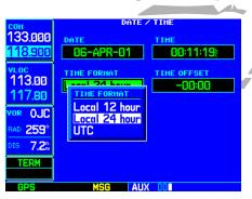
STEP 2 & 3 (top): Rotate the **small right knob** to select the desired time format.
