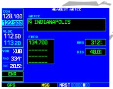
To scroll through the ARTCC or FSS frequencies, highlight the number adjacent to the communication point name and rotate the **small right knob**.
