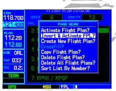
"Activate Flight Plan?" selects the highlighted flight plan and uses it for navigation guidance. "Invert & Activate FPL?" reverses the order of waypoints in the flight plan, then selects it for navigation guidance.
