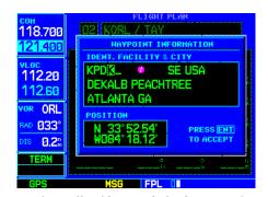
Use the **small** and **large right knobs** to enter the identifier of each flight plan waypoint.
