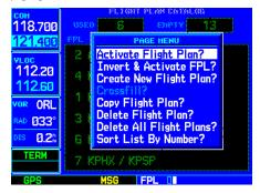
"Activate Flight Plan?" selects the highlighted flight plan for navigation guidance. "Invert & Activate FPL?" reverses the sequence of the highlighted flight plan, then activates it for navigation guidance.
