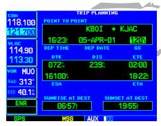
The Trip Planning Page calculates desired track, distance, estimated time en route, en-route safe altitude and estimated time of arrival for a specified direct-to, point-to-point or flight plan.
