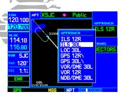
STEP 3 & 4: With the cursor on the "APPROACH" name field, rotate the **small right knob** to select the desired procedure and press **ENT**.
