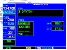
STEP 3 & 4: Rotate the **small right knob** to select the desired FSS, then rotate the **large right knob** to highlight the desired frequency.
