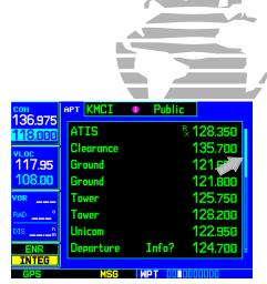
Whenever the GNS 530 is displaying a list of information that is too long for the display screen, a scroll bar appears along the right-hand side of the display. The scroll bar graphically indicates the number of additional items available within the selected category.
