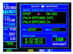
The "CRS" field allows you to define the course to a direct-to destination waypoint. Use the **small** and **large right knobs** to enter the desired course.
