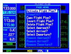
Select "Activate Flight Plan?" from the page menu to begin using the new flight plan.
