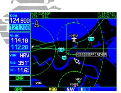
The Map Page can be used to create a user waypoint, by panning to the desired location and pressing **ENT**.
