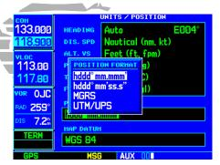
STEP 3 (top): Rotate the **small right knob** to select the desired position format.
