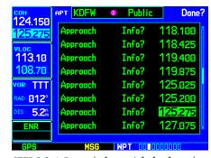
STEP 3 & 4: Rotate the **large right knob** to select the desired frequency. Press **ENT** to place the frequency on standby.
