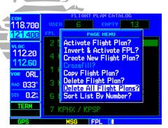
Select "Delete Flight Plan?" to remove the highlighted flight plan from memory. "Delete All Flight Plans?" removes all flight plans from memory.
