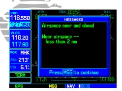
Press **MSG** to view an airspace alert message. Press **MSG** again to remove the message window and return to the previous page.
