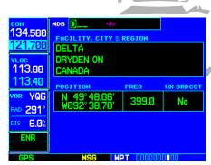
To display information for an NDB, highlight the identifier field. Then use the **small** and **large right knobs** to enter the NDB's identifier.
