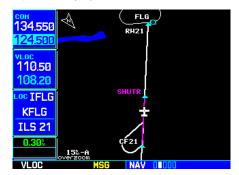
"VLOC" must appear in the lower right corner (above the **CDI** key) in order to use the VLOC receiver with your external CDI and autopilot.
