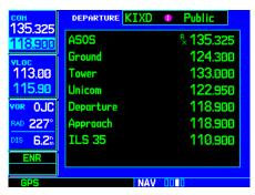
Once the standby frequency is selected, use the **COM flip-flop** key to make the frequency active for transmit and receive operations.
