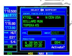
STEP 1: Press **direct-to** and select "KTOP" as your destination (using the **small** and **large right knobs**).
