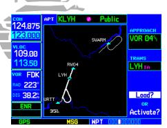
When an approach is "Loaded", it is added to the end of the active flight plan. Prior to reaching the approach course, select "Activate Approach?" to begin navigation along the approach course.
