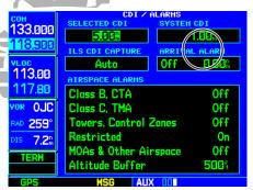
STEP 3 (top): The "System CDI" field indicates the current CDI scale in use. This setting may be lower than the "Selected CDI" setting when necessary for the current phase of flight — such as during an approach.
