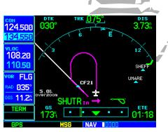
The GNS 530 can use its internal GPS receiver to guide you on the initial portion of an ILS approach. At this stage "GPS" is indicated above the **CDI** key.
