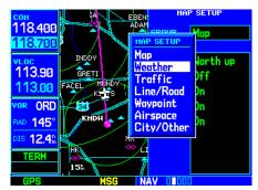
\* Weather and Traffic settings are only available when the GNS 530 installation includes connection to traffic and/or weather information sources. See 400/500 Series Display Interfaces Pilot's Guide Addendum.
