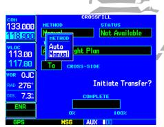
STEP 2: From the METHOD field, rotate the **small right knob** to select "Auto" or "Manual". "Auto" automatically transfers direct-to or active flight plan selections between units.
