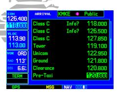
The scroll bar along the right-hand side of the page indicates the length of the NAVCOM frequency list and what portion of the list is currently being displayed.
