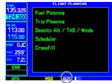
...then, rotate the **large right knob** to select the AUX page group, as indicated by "AUX" at the bottom of the screen. Rotate the **small right knob** to select the desired page within the group.
