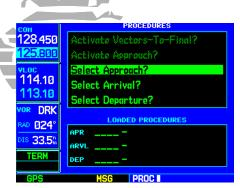
STEP 2: Once the destination airport is selected (using direct-to or an active flight plan), press **PROC** and choose the "Select Approach" option.
