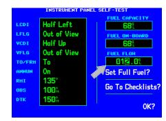
Enter the fuel capacity, fuel on board or fuel flow figures directly onto the appropriate field of the Instrument Panel Self-Test Page. Fuel on board and fuel flow are automatically provided if your installation includes connection to external sensors.
