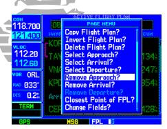
Approaches, arrivals and departures can all be removed from the active flight plan by selecting the corresponding "Remove..." option.
