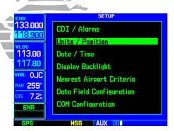
STEP 2: From the Setup Page, highlight the desired menu option and press **ENT**...
