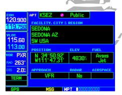
When a single waypoint is displayed on-screen, select it as your destination by pressing **direct-to**. When a list of waypoints is displayed, press the **small right knob** to display a cursor, highlight the desired waypoint, then press **direct-to**.
