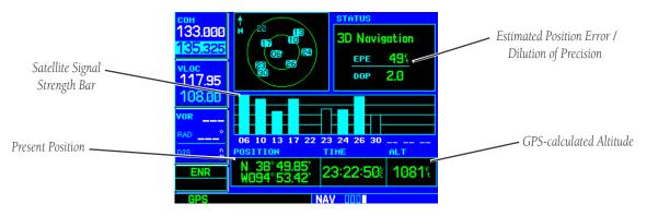
As the GPS receiver locks onto satellites, a signal strength bar appears for each satellite in view, with the appropriate satellite number (01-32) underneath each bar. The progress of satellite acquisition is shown in three stages:
