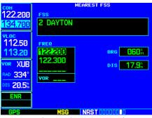
STEP 5 & 6 (next page): Press **ENT** to place the frequency on standby. Press the **COM** or **VLOC flip-flop** key to activate the selected frequency. Navigation frequencies for ILS and localizer (LOC) also appear on the list.
