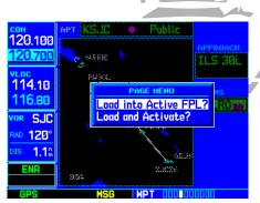
STEP 2 & 3: From the Airport Approach Page, press **MENU** to display an options list. Select "Load into Active FPL?" to load the approach for later use.
