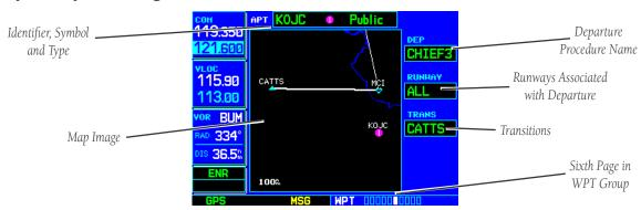
The Airport Departure Page shows the available Airport Departure Procedures (DPs; also referred to as SIDs) for the selected airport. Where multiple runways or transitions are associated with the departure procedure, that information may also be displayed. A map image provides a layout diagram for each departure, runway and transition.
