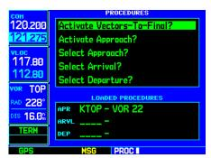
STEP 4 (bottom): Press **PROC** and select "Activate Vectors-To-Final?" to activate only the final course segment of a loaded approach.
