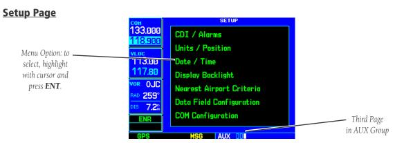
The Setup Page provides access (via a list of "menu options") to airspace alarms, CDI scale adjustments, an arrival alarm, units of measure settings, position formats, map datums, settings for local or UTC time display, display adjustments, nearest airport search parameters, data field configurations and COM transceiver channel spacing. When a menu option is selected, the corresponding page appears providing access to the various unit settings.
