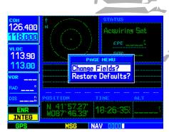
By default, current altitude (ALT) is displayed in the lower right corner of the page. This field is user selectable using the "Change Fields?" option.
