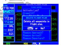
"Delete Flight Plan?" cancels navigation and removes the active flight plan from memory.
