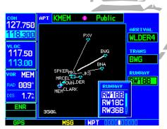
STEP 7: With the "RUNWAY" field highlighted, rotate the **small right knob** to select the desired runway. Many arrivals apply to all runways for a particular airport, as indicated by "ALL".
