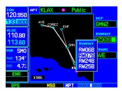
STEP 5: With the cursor on the "RUNWAY" field, rotate the **small right knob** to display a list of available runways.
