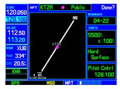
STEP 5: To display additional database information, press the **small right knob** to remove the cursor, then rotate the **small right knob** to select the desired page.
