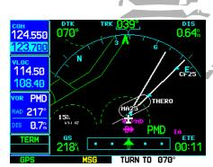
STEP 1: As the distance to the IAF approaches zero, the waypoint alert is replaced by a turn advisory ("TURN TO 070°"). Initiate a standard rate turn to this course heading.
