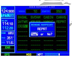
STEP 3 & 4 (bottom): From the User Waypoint List, use the **small** and **large right knobs** to rename an existing waypoint. Press **ENT** to display a "Rename Waypoint" confirmation window.
