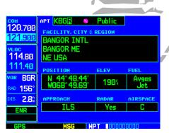
Enter a waypoint identifier on the top line of any WPT page (using the **small** and **large right knobs**). Once entered, the database information for the selected waypoint is displayed.
