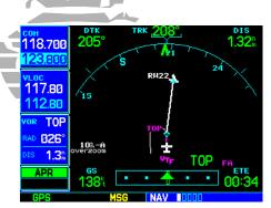
STEP 6: At 2.0 nautical miles from the FAF, the GNS 530 switches from terminal ("TERM") to approach ("APR") mode. The CDI scale transitions from 1.0 to 0.3 nautical mile, full scale.
