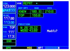
STEP 5: Use the **small** and **large right knobs** to enter the radial from the reference waypoint to the new user waypoint.
