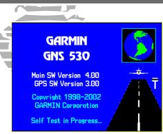
The Welcome Page appears when the GNS 530 is powered on. During the time this screen is displayed, the GNS 530 performs a self test to ensure proper operation.
