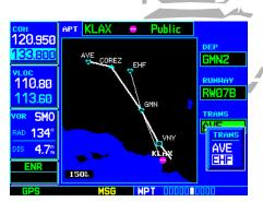
STEP 7: With the "TRANS" field highlighted, rotate the **small right knob** to select the desired transition.
