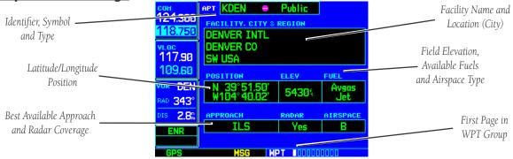
The Airport Location Page displays the latitude, longitude, and elevation of the selected airport. The Airport Location Page also displays facility name and location, as well as fuel availability, best available instrument approach, radar coverage and airspace type. The following descriptions and abbreviations are used:
