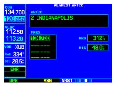
STEP 5 & 6: Press **ENT** to place the frequency on standby. Press the **COM flip-flop** key to activate the selected frequency.
