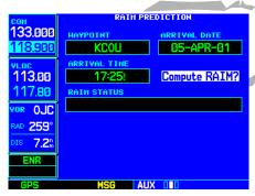
STEP 5: Once the destination, date and time are entered, select "Compute RAIM?" to determine if satellite coverage is adequate for the flight.
