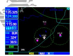
Press the **small left knob** to move the tuning cursor to the VLOC window. Rotate the **small left knob** to select the kilohertz portion of the frequency and the **large left knob** to select the megahertz portion.
