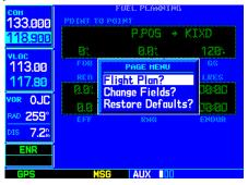
STEP 2 & 3c: For "flight plan leg" fuel planning, select "Flight Plan?" from the options window. Use the **small right knob** to select the desired flight plan and the desired leg of the flight plan.
