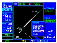
STEP 3: Once the approach is selected (by name), a pop-up window asks you to select the appropriate transition ("SHUTR" intersection, in this example).
