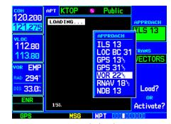
STEP 2: Press **PROC** and select the "VOR 22" approach and "D258G" transition (using the **large right knob** and **ENT**).
