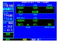
Select the "Density Alt / TAS / Winds" option to calculate density altitude, true airspeed and winds aloft.
