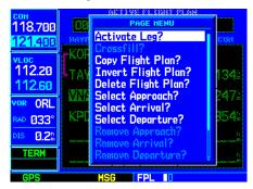
"Activate Leg?" selects the highlighted flight plan leg as the leg currently in use for navigation guidance (even if it isn't the closest leg).
