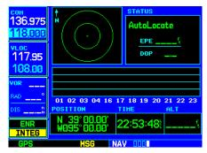
"AutoLocate" appears when the GNS 530 has orbital data, but last known position and/or time information are significantly different from current conditions
