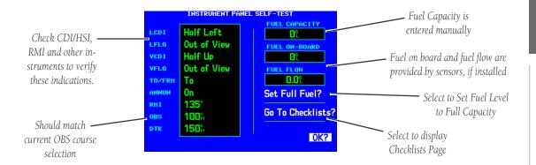
Once the database has been acknowledged, the Instrument Panel Self-Test Page appears. To ensure that your GNS 530 and any connected instruments are working properly, check for the following indications on your CDI/HSI, RMI, external annunciators and other connected instruments:
