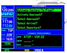
STEP 2: If the approach is loaded, but not yet activated, press **PROC** and select "Activate Vectors-To-Final?".
