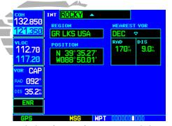
To display information for an intersection, highlight the identifier field. Then use the **small** and **large right knobs** to enter the intersection name.
