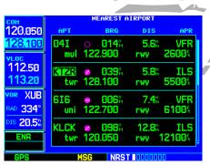
STEP 3 & 4: Highlight the identifier of the desired airport and press **ENT** to display the database information — beginning with location and fuel.
