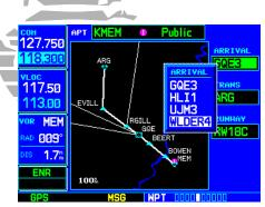
STEP 2 & 3: With the cursor on the "ARRIVAL" field, rotate the **small right knob** to display a list of available arrival procedures.
