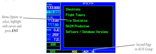
The Utility Page provides access (via a list of "menu options") to checklists, a count down/up timer, trip timers, trip statistics, RAIM (Receiver Autonomous Integrity Monitoring) prediction and software/database version information. When a menu option is selected, the corresponding page appears providing additional information and features.
