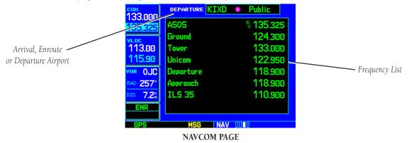
A frequency listed on the NAVCOM Page can be quickly transferred to the standby field of the COM or VLOC windows. This time saving process prevents having to "re-key" a frequency already displayed elsewhere on the screen.
