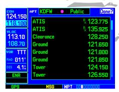
STEP 2: Highlight "View Frequencies?" and press **ENT** to display the communication frequency (s) for the controlling agency.
