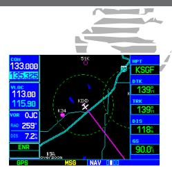
By adding data fields along the right-hand side, the Map Page can combine a moving map display and navigation data for complete situational awareness. Map setup pages are provided to add these data fields and to designate the maximum scale at which each map feature appears. These settings provide an automatic decluttering of the map (based upon your preferences) as you adjust the scale.
