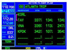
The Active Flight Plan Page shows waypoint names and data for the route currently being used for navigation guidance.
