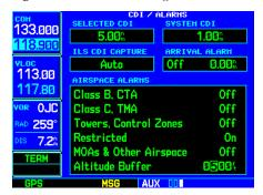
STEP 4: Use the **small** and **large right knobs** to enter the desired altitude buffer. This buffer distance is added to the floor/ceiling limits and provides an added margin of safety.
