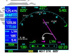
STEP 7 & 8: Procedure turn, inbound. The CDI needle swings to the opposite side for proper sensing and "NEXT DTK 025°" appears. Turn to the new heading as the needle begins to center.
