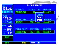
STEP 3 (top): Rotate the **small right knob** to select a count "Down" or count "Up" timer.
