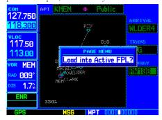
STEP 2 & 3: From the Airport Arrival Page, press **MENU** to display an options list. "Load into Active FPL?" allows you to add the arrival procedure to your flight plan for later use.
