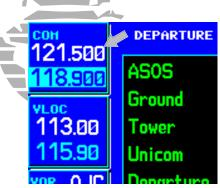
Press and hold the **COM flip-flop** key for two seconds to activate the 121.500 MHz emergency frequency.
