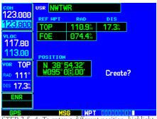
STEP 3 & 4: To enter a different position, highlight the position field and use the **small** and **large right knobs** to enter the new position coordinates.
