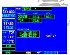
STEP 3 & 4: Use the **small** and **large right knobs** to enter the name of the reference waypoint. Press **ENT** and the cursor moves to the radial (RAD) field.
