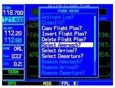
Published instrument approaches can be selected and used from the Active Flight Plan Options, or by pressing the **PROC** key. The "Select Approach?" option appears in both places.
