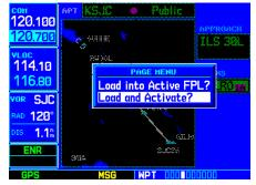
Select "Load and Activate?" to immediately begin using the approach waypoints for navigation guidance.
