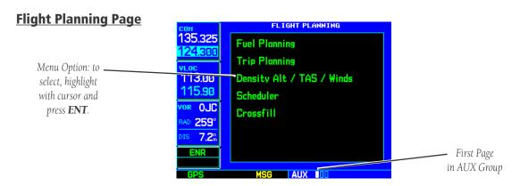
The Flight Planning Page provides access (via a list of "menu options") to E6B functions for fuel planning, trip planning, density altitude/true airspeed/winds aloft calculations, scheduled messages and a "Crossfill" function to transfer flight plans/user waypoints to a second GNS 530. When a menu option is selected, the corresponding page appears providing additional information and features.
