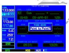
STEP 2: Press **MENU** and use the options window to select the other leg mode: Point-to-Point or Flight Plan.
