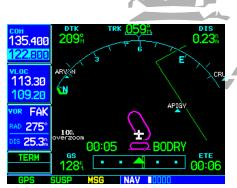
STEP 9: While flying the holding pattern, a timer appears on the Default NAV Page. Use the timer to fly the one minute outbound portion of the pattern.
