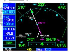
STEP 9: The GNS 530 automatically switches from the GPS receiver to the VLOC receiver as you complete the turn inbound. The annunciator above the **CDI** key switches from "GPS" to "VLOC".
