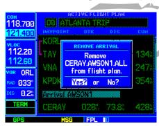
To remove an approach, departure or arrival from the active flight plan, highlight the procedure name (appears in light blue text) and press **CLR**.
