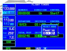
STEP 3 (top): Rotate the **small right knob** to select when the trip timer resets: each time the GNS 530 is powered on or when ground speed exceeds 30 knots.
