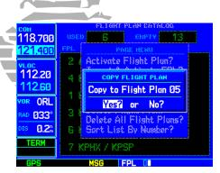
Use the "Copy Flight Plan?" option to save a copy of a flight plan to another memory location. This is useful for saving the active flight plan, or to save a stored flight plan before editing.
