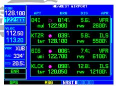
STEP 2 (top): Rotate the **large right knob** to select the NRST page group. "NRST" appears at the bottom of the screen.
