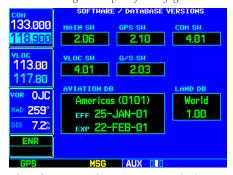
The Software / Database Versions Page displays the internal software versions for the GNS 530's various subsystems as well as the Jeppesen database and built-in land data.
