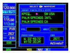
Use the **small** and **large right knobs** to enter the name of the destination waypoint. Press **ENT** once the name has been fully entered.
