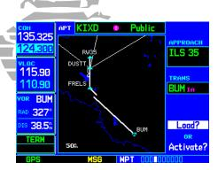
STEP 6 & 7: Select "Load?" or "Activate?" and press **ENT**. Verify that the navigation frequency is automatically placed on standby. To activate the frequency, press the **VLOC flip-flop** key.
