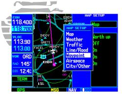
To select a map setup group, rotate the **small right knob**. Rotate the **large right knob** to highlight the desired setting within the group.
