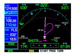
STEP 7: "START PROC TRN" appears in the lower right corner of the screen to remind you to initiate the procedure turn.
