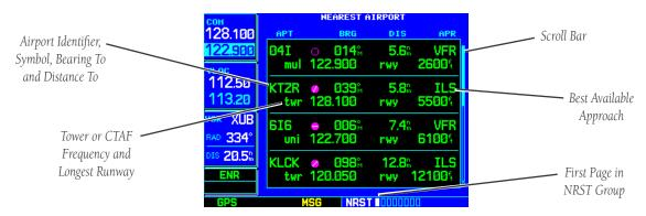
The Nearest Airport Page may be used to quickly tune the COM transceiver to a nearby airport. The selected frequency is placed in the standby field of the COM window and activated using the **COM flip-flop** key.
