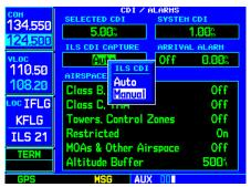
If the ILS CDI Capture setting is changed to "Manual", you must select VLOC guidance manually by pressing the **CDI** key.
