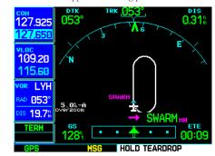
STEP 3: An alert message in the lower right hand corner recommends entry procedures for the holding pattern (e.g, "HOLD TEARDROP").
