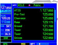
When the frequency list is too long to display on a single page, the scroll bar along the right-hand side of the list indicates the portion of the list that you are currently viewing (the shaded area) and the overall length of the list (indicated by the height of shaded and unshaded areas).
