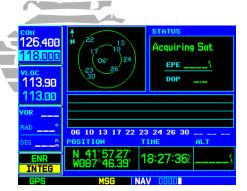
When the GNS 530 is first powered on, an "Acquiring" status appears at the top of the page and no signal strength bars are displayed.
