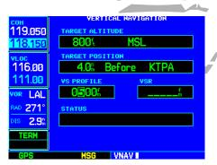
STEP 8: The default profile is a 400 foot-per-minute climb/descent. Use the **small** and **large right knobs** to enter a different vertical speed figure.
